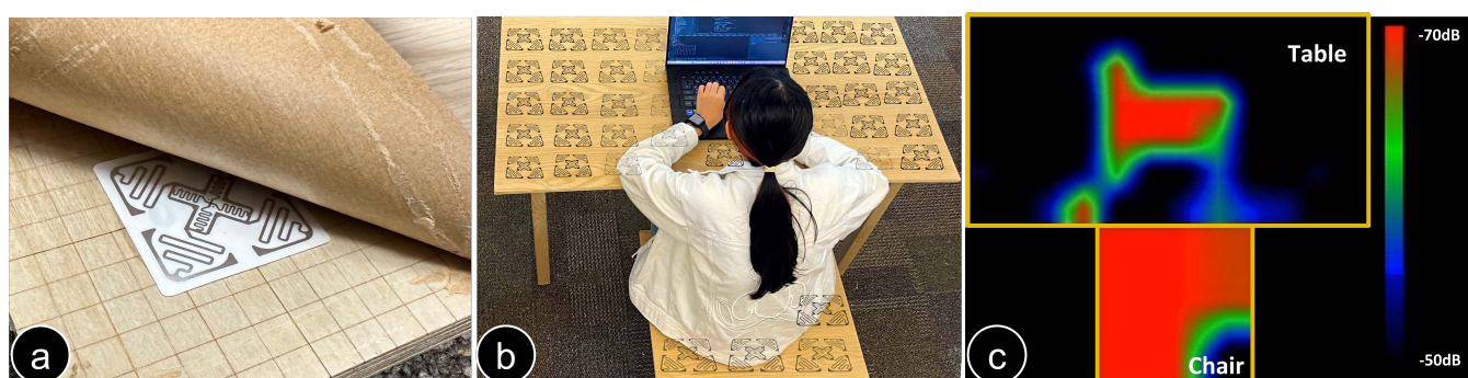
Figure 1: (a) Tagnoo is a computational plywood, consisting of a plywood panel augmented with a grid of RFID tags. (b) Tagnoo can be used to construct office furniture like a table and chair, which are capable of sensing the presence of an object or user. (c) The heatmap image of the RSSI values captured while a user is seated at a desk using a laptop. The upper segment shows the sensor data obtained from the desk, while the lower segment shows the sensor data obtained from the chair.
